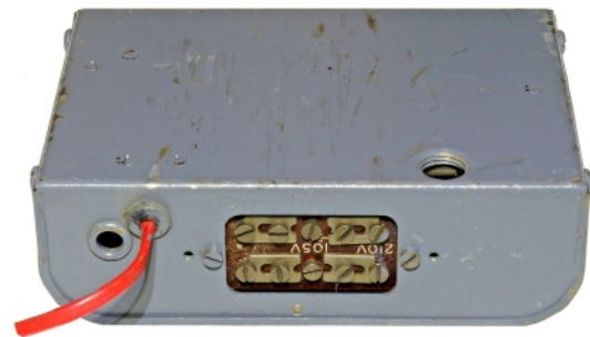
View of voltage selector panel with range plunger stowage (above); with cover opened showing the miniature mains transformer and rectifier valve 3A5 (below).
