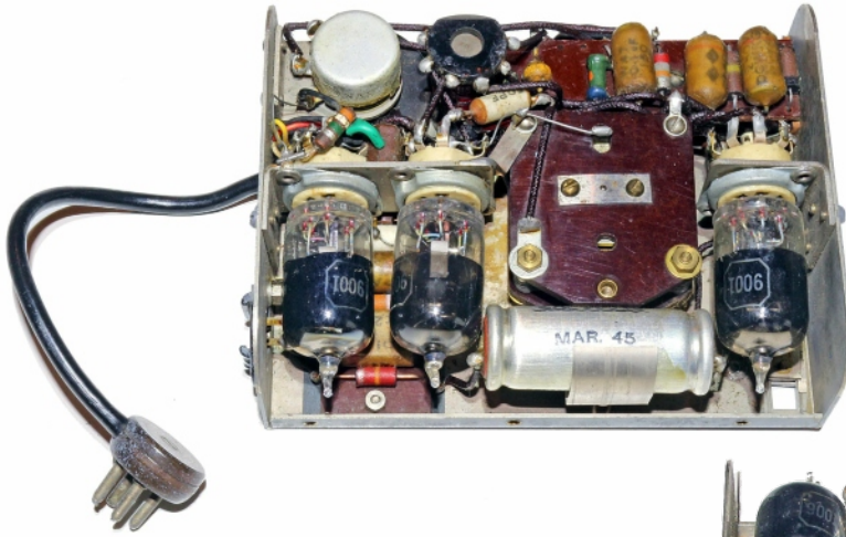
Inside view of Receiver Type 53/1 showing the very compact build with its three 9001 valves, tuning condenser C7 and tuning coil L2/3/4. Note the production date stamp March 1945 on the electrolytic condenser C13.
